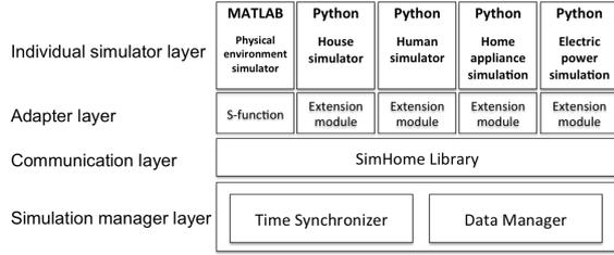
Figure 1: The examples of layered architecture of physical environment simulator
