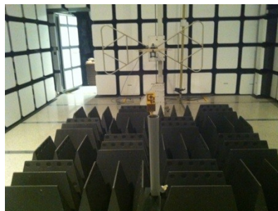
Fig. 3: Measurement using a vector network analyzer in an anechoic chamber
