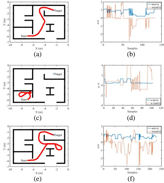
Fig. 9. The path and velocity responses of robot in three architectures in Case 2: (a) and (b): BBFM, (c) and (d): MOASM, (e) and (f): CDB
