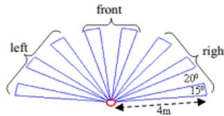
Fig. 4: Arrangement of ultrasonic sensors on the robot.
