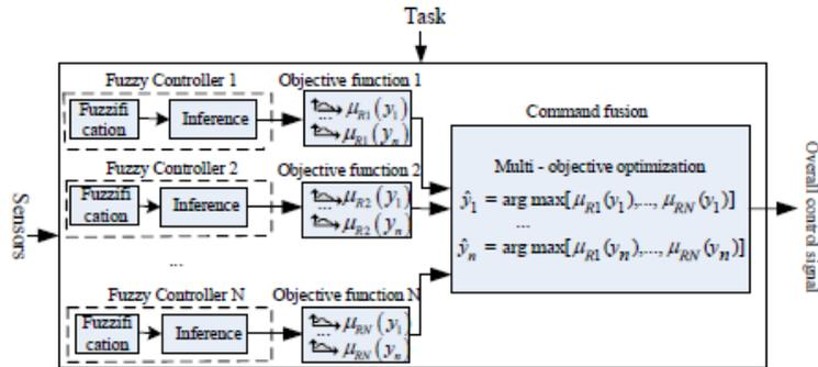
Fig. 2. The block diagram of BBFM architecture.
