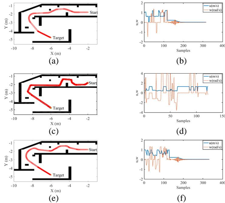
Fig. 9. The path and velocity responses of robot in three architectures in Case 2: (a) and (b): BBFM, (c) and (d): MOASM, (e) and (f): CDB.
