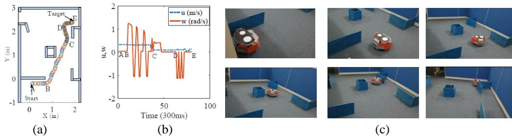
Fig. 11. The results of navigating operations: (a) Path, (b) Velocity responses, (c) Photos.
