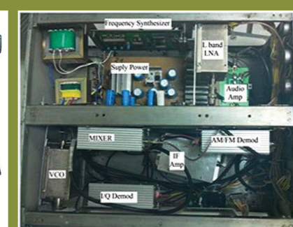
A3: Completed structure of L-band receiver
