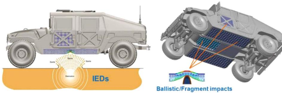
Fig. 1. An application of lightweight auxetic composite plate to enhance the ballistic and impact resistance capabilities of armoured vehicles [1].
