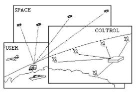
Figure 3. Structure of the GPS
