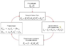
Figure 4. Kalman Filter loop
