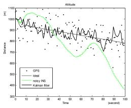
Figure 10. Altitude of the aircraft in case deviation of the GPS is increased.
