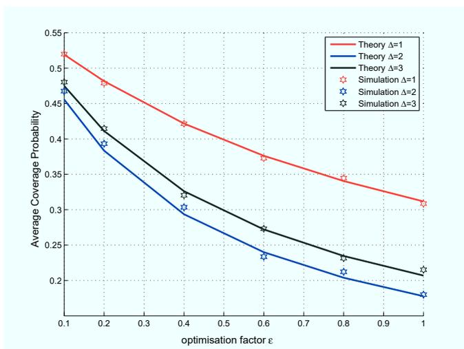
Fig. 3. Average coverage probability with different values of frequency reuse factor  $\Delta$
