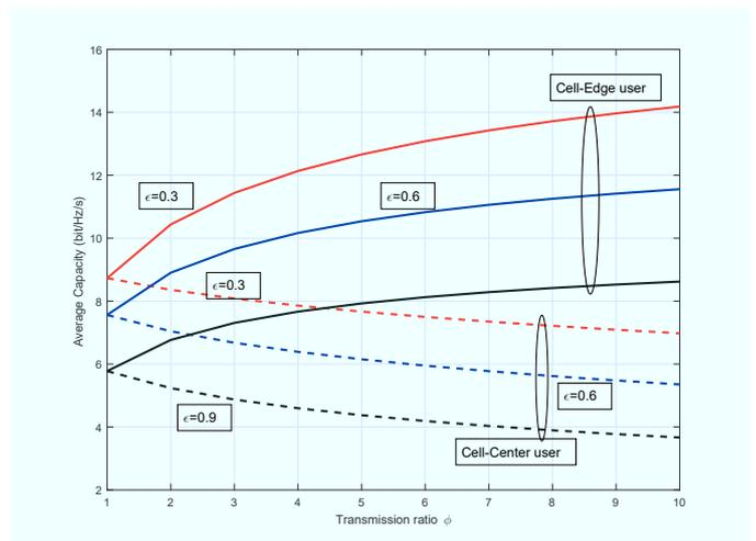
Fig. 4. Average capacity with different values of the power ratio  $\phi$
