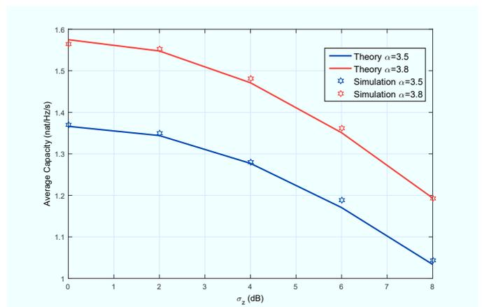
Fig. 5. Capacity with different values of path loss exponent  $\alpha$  and Rayleigh-Lognormal variance  $\sigma_z$
