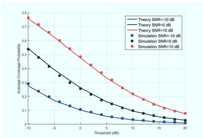
Fig. 2. Coverage probability with different values of SNR and the threshold  $T$
