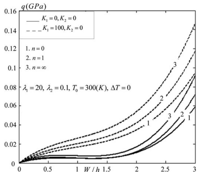
**Figure 5.** The effects of the volume fraction index  $n$  and elastic foundation on the nonlinear response of S-FGM SS shells under uniform external pressure.
