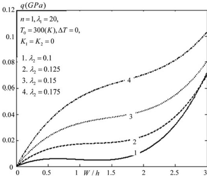
**Figure 6.** The effects of radius ratio  $H/a$  on the nonlinear stability of S-FGM SS shells under uniform external pressure without an elastic foundation.
