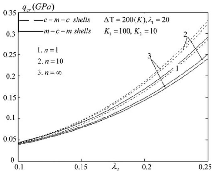
**Figure 14.** The effects of the volume fraction index  $n$  on the critical buckling pressures of the shells.
