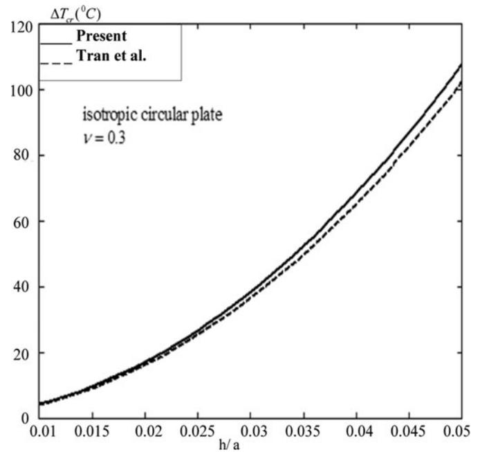
Figure 2. Comparison of the critical buckling temperature change for clamped isotropic FGM circular plate under uniform temperature rise.
