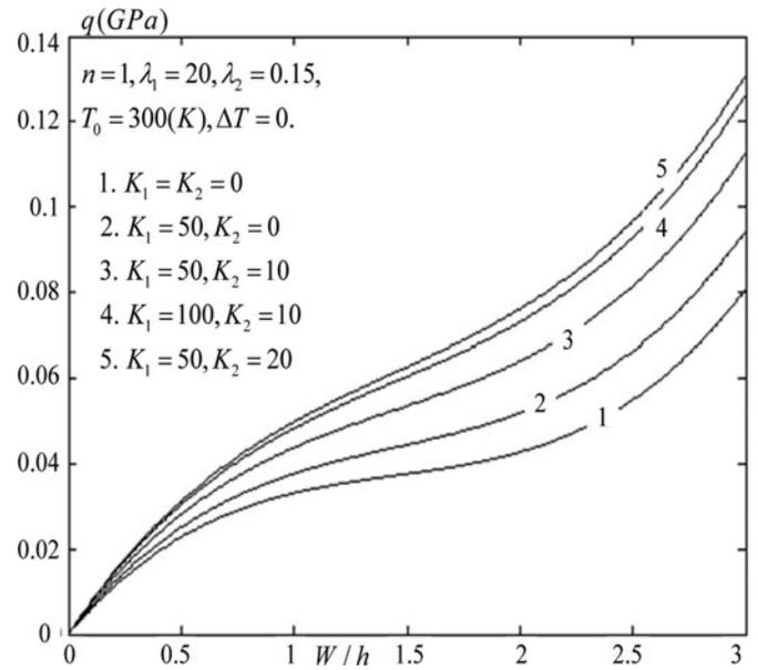
**Figure 8.** Effects of nondimensional stiffness parameters  $K_1, K_2$  on the nonlinear response of S-FGM SS shells.
