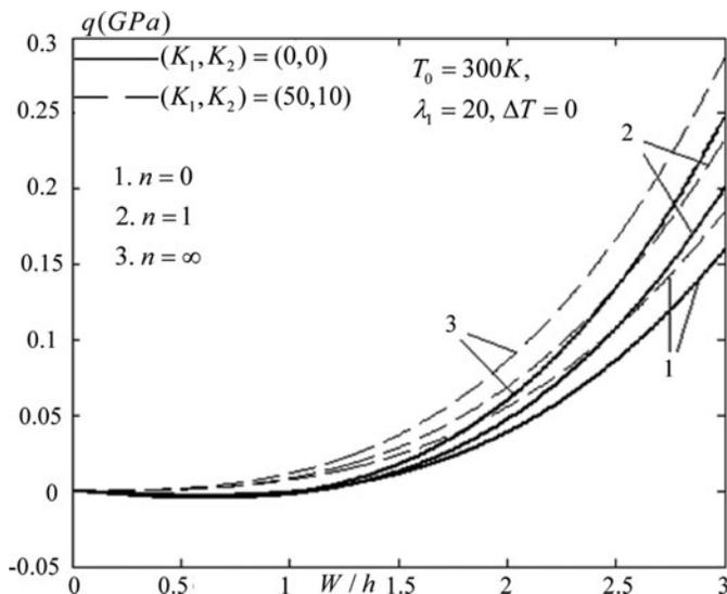
Figure 11. Effects of material distribution and foundation stiffness on the nonlinear response of S-FGM circular plates under uniform external pressure.
