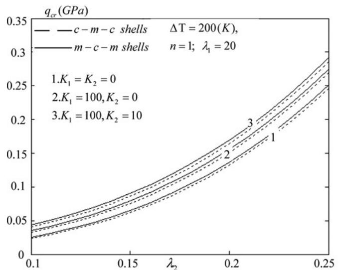
Figure 13. The effects of nondimensional stiffness parameters  $K_1, K_2$  on the critical buckling pressures of the shells.
