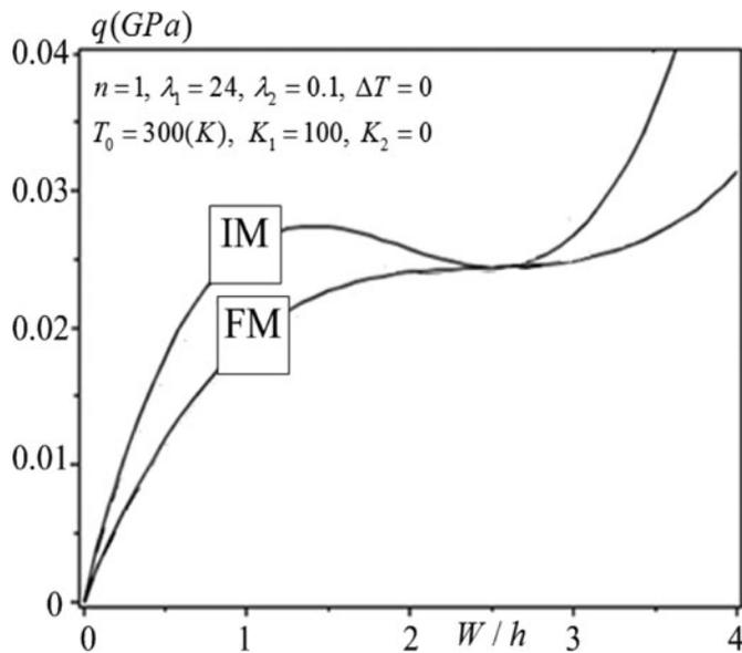
**Figure 15.** The effects of in-plane restraint conditions on the nonlinear response of the shell.
