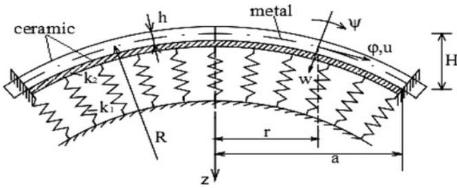
**Figure 1.** Configuration and the coordinate system of an S-FGM shallow spherical shell (S-FGM SS shell).
