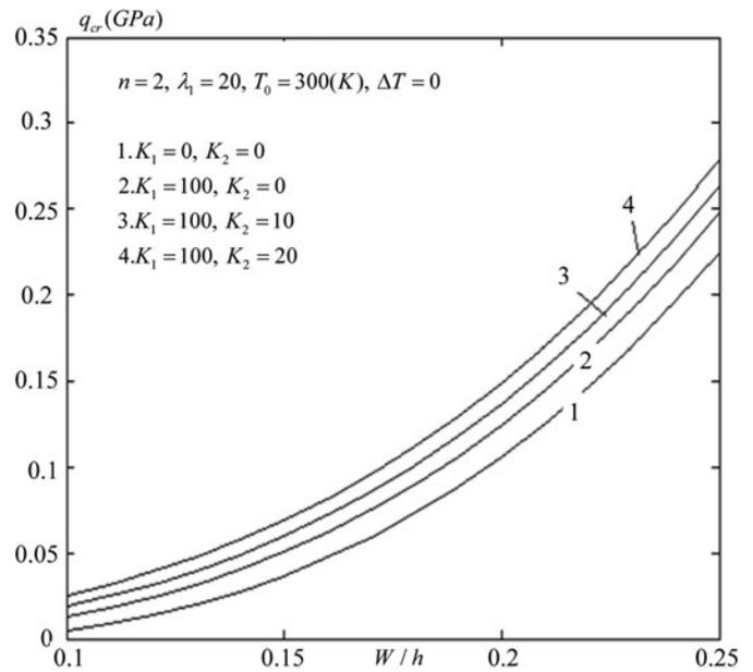
**Figure 4.** Effects of stiffness parameters of elastic foundations on the critical buckling pressure of the S-FGM SS shell.
