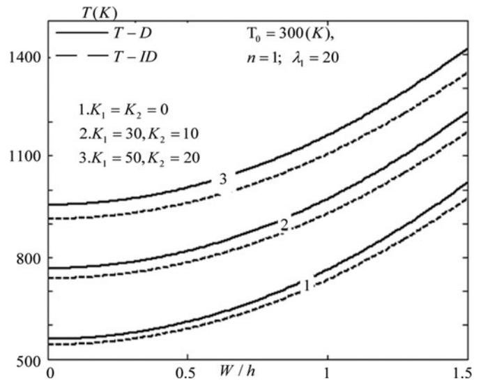
Figure 12. Effects of elastic foundations and temperature dependent properties on the thermal post-buckling of the S-FGM circular plates.
