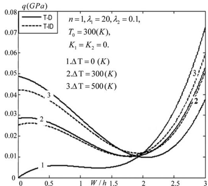
**Figure 9.** Effects of thermal environments on the nonlinear thermo-mechanical response of S-FGM SS shells.
