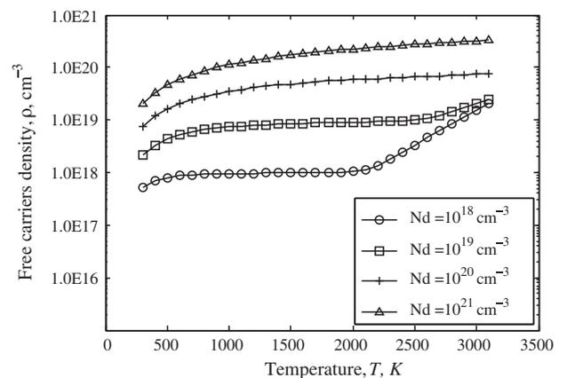
Fig. 3. Plot of free charge carrier concentration as a function of temperature at different level of doping concentration.
