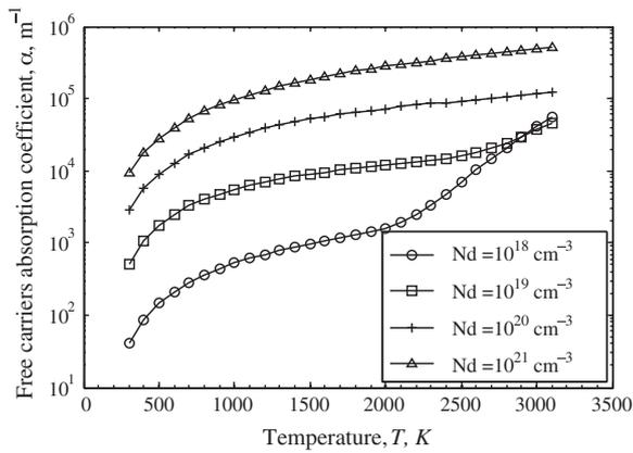
Fig. 4. Plot of free charge carrier absorption coefficient as a function of temperature at different level of doping concentration.
