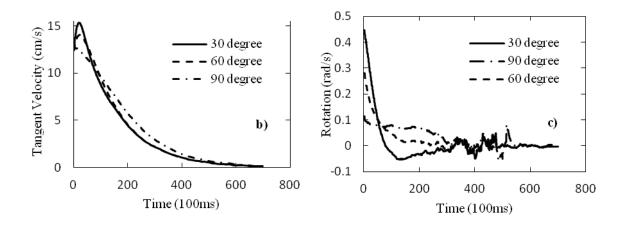
*Figure 7.* Results of stabilization control: a) Trajectories of the robot b) Tangent velocity c) Direction variation
