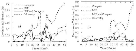
*Figure 5.* The deviation in X and Y direction between estimated positions and the real one a) Deviation in X direction b) Deviation in Y direction
