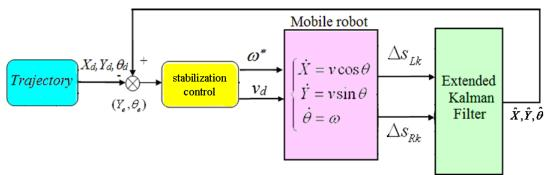
Figure 2. The control model
