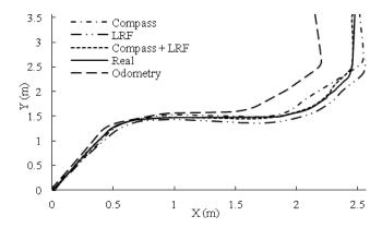
Figure 4. Estimated robot trajectories under different EKF configurations [27]
