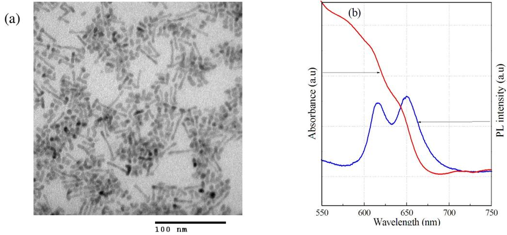
Figure 7. TEM images (a) and absorption, PL (b) of CdSe/CdSe<sub>1-x</sub>S<sub>x</sub> nanorods samples kept in the OLA solution at 80°C for 12 hours.
