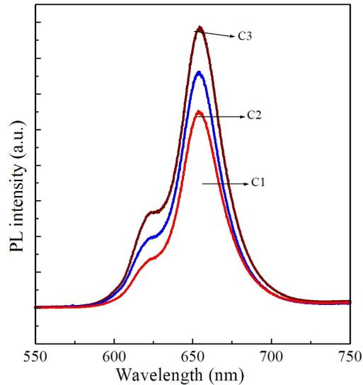
Figure 8. PL peak intensity of NHS CdSe/CdSe<sub>1-x</sub>S<sub>x</sub> nanorods obtained by size- selective centrifugation.
