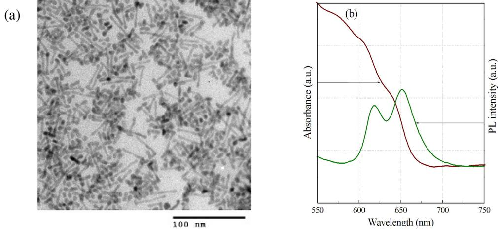
Figure 6. TEM images (a) and absorption, PL spectra (b) of CdSe/CdSe<sub>1-x</sub>S<sub>x</sub> nanorods were synthesized with OLA 30 % mixed in the reaction solution.
