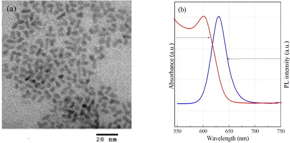
Figure 3. TEM images (a), and absorption and PL of CdSe NCs (b), were synthesized in the mixed solutions of ODE-OA-TOP using TOPO and OLA at temperature of 250°C.
