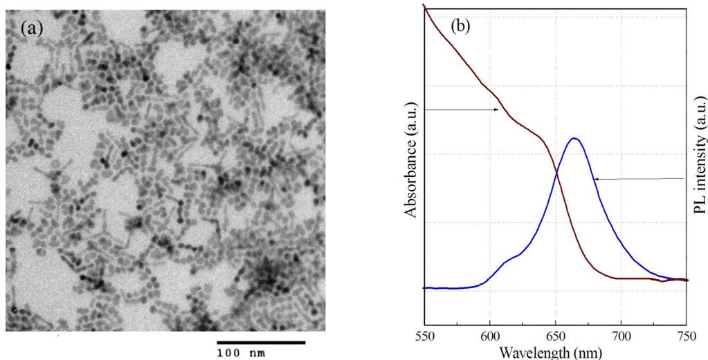
Figure 5. TEM images (a) and absorption, PL spectra (b) of CdSe/CdSe<sub>1-x</sub>S<sub>x</sub> nanorods were synthesized with OLA 5% mixed in the reaction solution.
