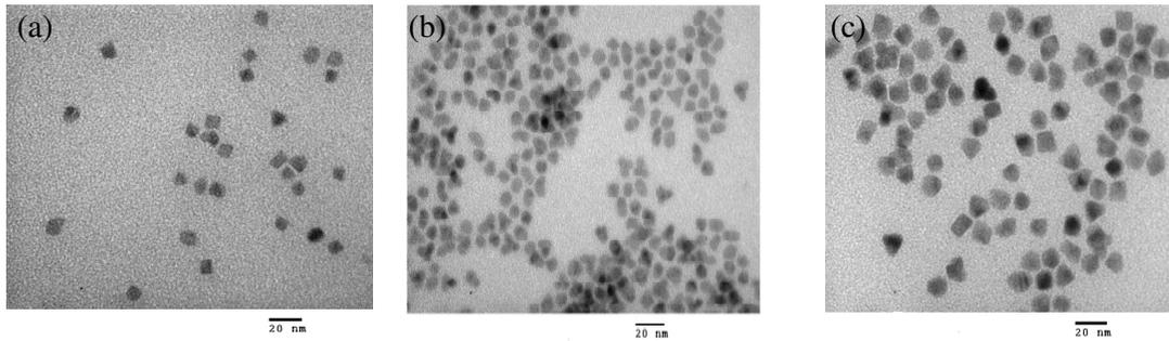
Figure 1. TEM images of CdSe NCs were synthesized at different reaction temperature of a) 290°C , b) 300°C, c) 310°C in the ODE-OA-TOP reaction system.
