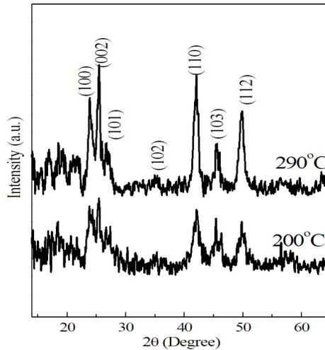
Figure 4. XRD patterns of CdSe NCs formed in the ODE-OA-TOP reaction system coupled with OLA/TOPO solution having the ratio of 3:1 and at reaction temperatures of 200°C and 290°C.
