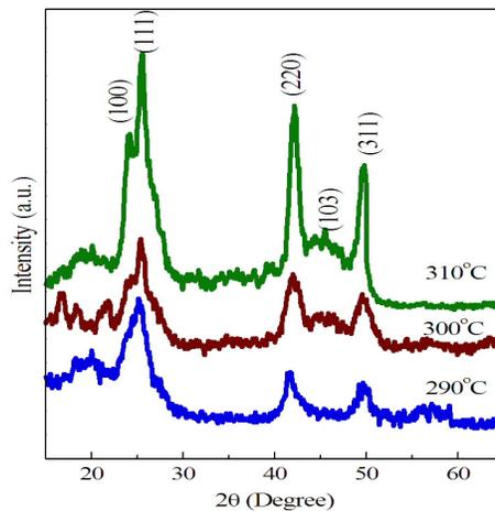
Figure 2. XRD patterns of CdSe NCs were synthesized at reaction temperature of 290° to 310°C in the ODE-OA-TOP reaction system.
