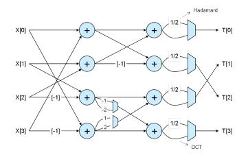
Figure 3. Hybrid 1-D transform architecture for integer DCT-based and Hadamard transforms.
