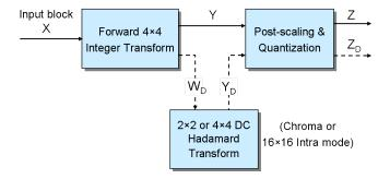
Figure 2. Transform and quantization flow diagram.
