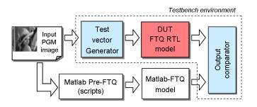
Figure 10. Verification model for the design.
