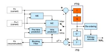
Figure 1. H264/AVC encoder - a functional architecture.
