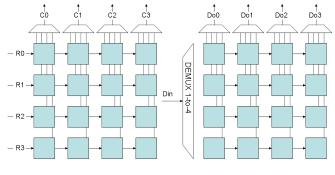
Figure 5. Transpose RAM (left) and DC RAM (right).
