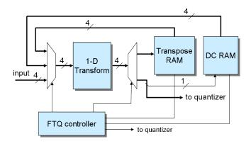
Figure 4. Architecture of forward transform.
