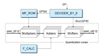
Figure 6. Quantizer architecture.
