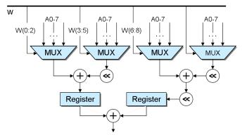
Figure 8. Multiplier for quantizer using the pre-multiplier element.
