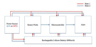
Figure 1. Block diagram of the device
