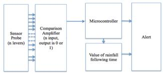
Figure 2. Electrode sensor interface with the MCU
