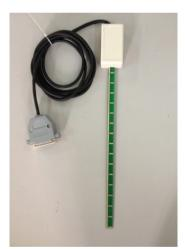
*Figure 3. Photo of an electrode sensor*
