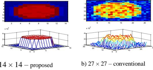
Fig. 5. Reconstruction of the object function after three iterations ( $N_1 = 14, N_2 = 27$ )
