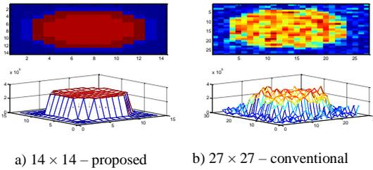
Fig. 6. Reconstruction of the object function after four iterations ( $N_1 = 14, N_2 = 27$ )
