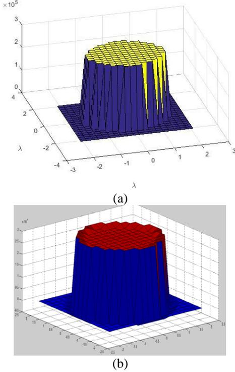
Fig 2. The difference between the object function for density imaging and sound contrast imaging.
