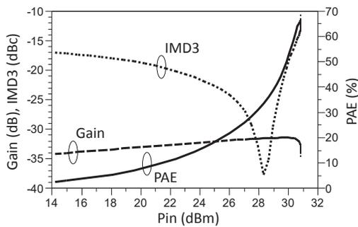
Fig. 11. Simulated two-tone results at 2.1 GHz and a spacing of 4 MHz.
