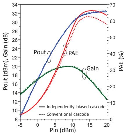
Fig. 12. Comparison of one-tone results between the independently biased cascode and the conventional one.
