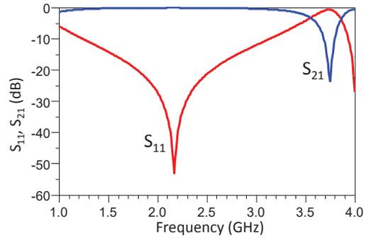
Fig. 4. Simulated S-parameters of the designed bias network.
