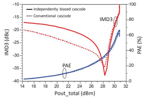
Fig. 13. Comparison of two-tone results between the independently biased cascode and the conventional one.
