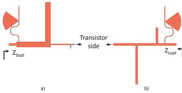
Fig. 6. EM model of the designed matching networks: a) Input matching network and b) output matching network.
