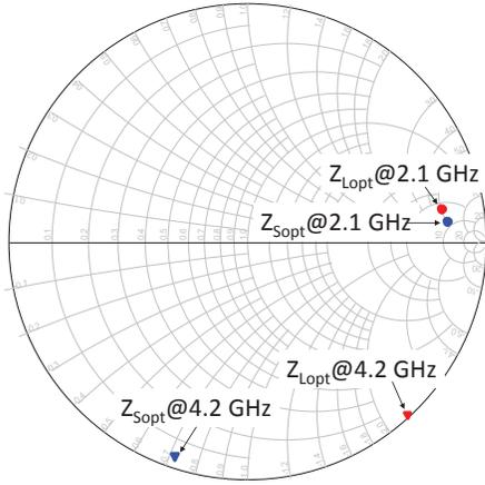
Fig. 2. Simulated optimum load and source impedances realized using load/source pull technique.
