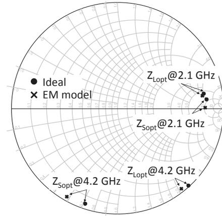
Fig. 7. Realization of the optimum impedances by the designed matching networks.
