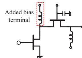
Fig. 1. Independently biased cascode configuration.
