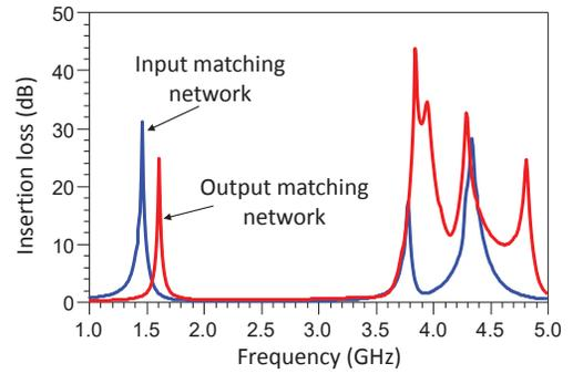
Fig. 8. Simulated insertion loss characteristic of the input/output matching network.
