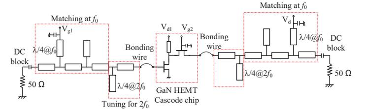
Fig. 9. Entire circuit schematic for co-simulation.
