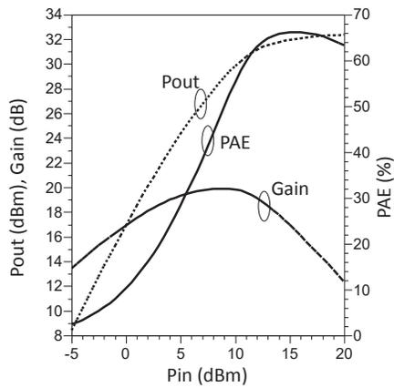
Fig. 10. Simulated one-tone results at 2.1 GHz.
