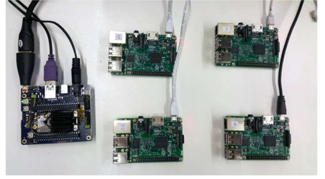
Fig. 8 Embedded IoT boards used for computer control
