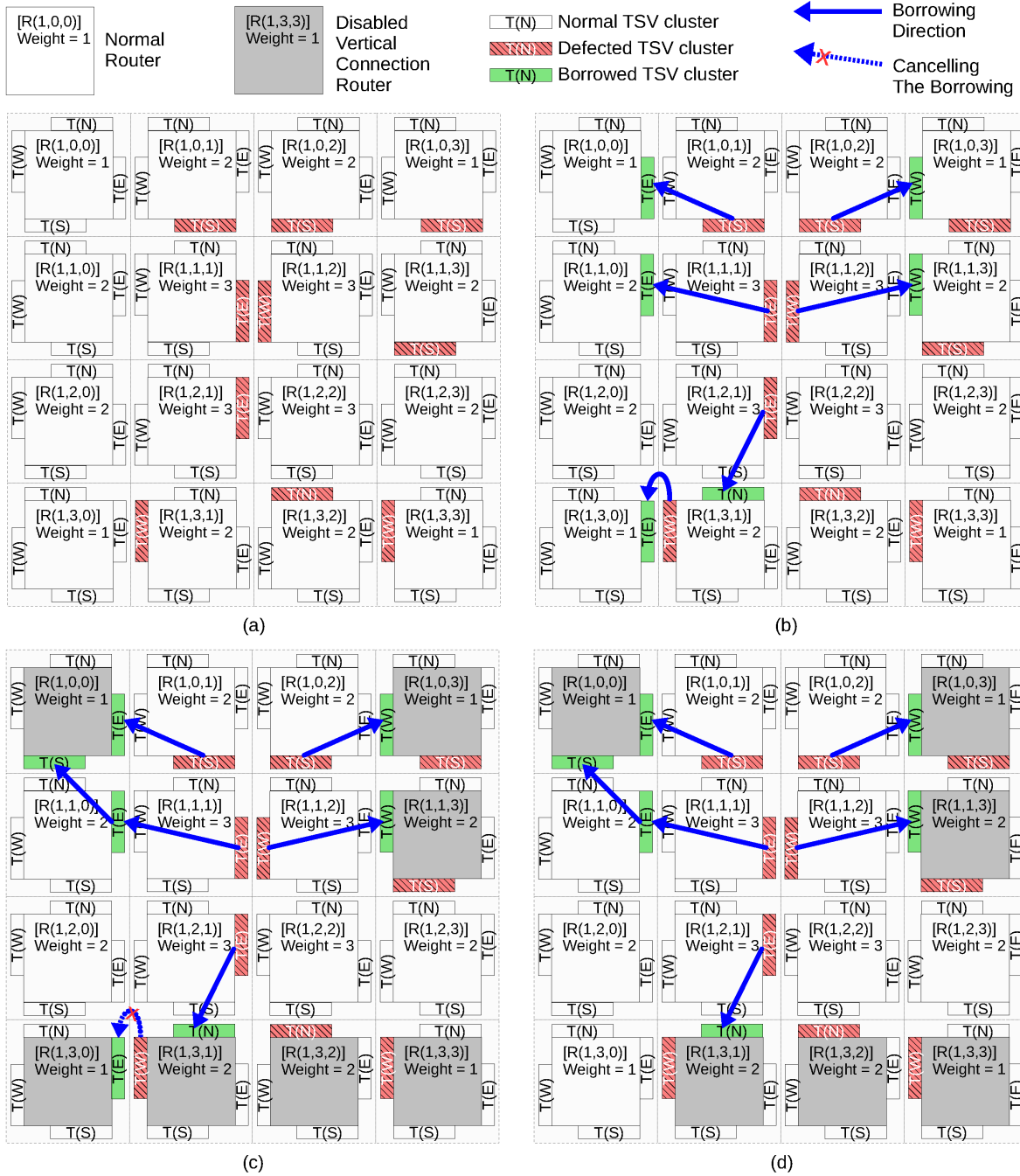
Fig. 5: An example of the sharing algorithm on a 4 \times 4 layer: (a) Initial state with ten defected TSV-clusters; (b) Best candidates selection; (c) Borrowing chain creating and selection refining. (d) Final result with six disabled routers.
