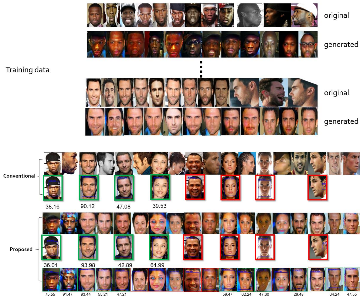
Figure 7. The results of the image generation from the training data set and comparison of the identification results between the conventional face recognition system and the proposed one using GAN.
