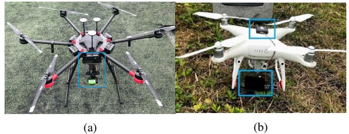
Fig. 2: Cameras and drones used. (a) Camera Sentera Quad Sensor installed on the drone DJI M600 Pro; (b) Camera MapIR Survey 3 installed on Phantom 4 Pro
