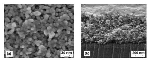
Fig. 1. FE-SEM bright-field micrograph of a doctor-blade deposited  $TiO_2$  film: surface view (a) and cross-section (b). The concentration of the colloidal solution was 5 wt.%  $TiO_2$  in water, and the spread speed was 8 mm/s. The thickness d of the film was about 550 nm.
