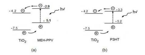
*Fig. 13. Band structure diagram illustrating the HOMO and LUMO energies of MEH-PPV (a) and P3HT (b) relative to the band structure of TiO<sub>2</sub>.*
