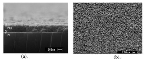
Fig. 4. SEM micrographs of a cross section of the annealed film (a) and surface morphology of the film. This clearly shows the submicro-structured grains of  $VO_2$  which were crystallized during the annealing. The thickness d = 240 nm.
