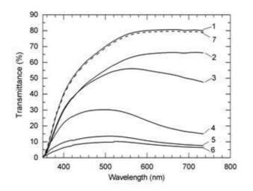
Fig. 2. In situ transmission spectra of the  $TiO_2/FTO$  colored in  $1M LiClO_4 + PC$  at -1.20 V/SCE versus time. The 1st curve is the transmittance spectra in open circuit; 2, 3, 4 and 5 - the spectra corresponding to respective coloration times of 0.5, 1, 1.5 and 2sec; 6 – saturated coloration state; 7 – completely bleached state.
