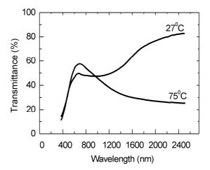
Fig. 6. Transmittance spectra of VO<sub>2</sub> film recorded at temperature lower  $\tau_c$  (top curve) and at temperature higher  $\tau_c$  (bottom curve).
