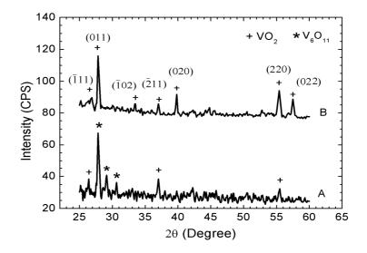
Fig. 3. XRD patterns of vanadium oxide films deposited by RF-sputtering followed by annealing. "A" patterns is of the film sputtered from  $VO_2$  target and "B" patterns – from  $V_2O_3$  target.
