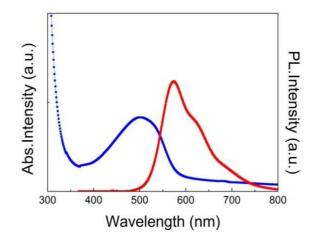
Fig. 8. Absorption and Photoluminescence spectra of MEH-PPV film.
