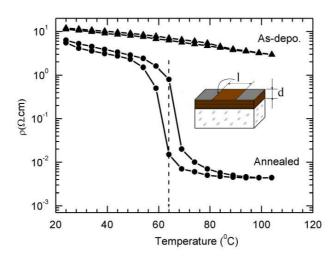
*Fig. 5. The temperature dependence of the resistivity of as-deposited film (top) and annealed film (bottom loop).*
