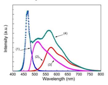
Fig. 9. Emission spectra of components of WLEDs made from nanocomposite: Blue LED (1), MEH-PPV (2), G-YAG:Ce nanopowder (3) and the total spectrum of the Blue LED, G-YAG:Ce and MEH-PPV (4).
