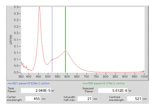
Fig. 10. Emission spectra of WLEDs made from by coating G-YAG and MEH-PPV hybrid composite onto InGaN blue chip.
