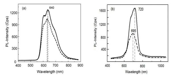
*Fig.* 12. (*a*): *PL spectra of MEH-PPV and MEH-PPV/nc-TiO*<sub>2</sub> (5 nm); (*b*): *P3HT and P3HT/nc-TiO*<sub>2</sub> (15 nm).
