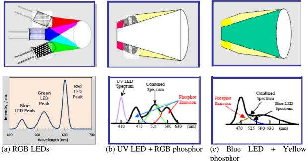
*Fig.* 7. *Three methods used for producing the white light LEDs: (a) - Red + Green + Blue LEDs, (b) - UV LED + RGB phosphor and (c) - Blue LED + Yellow phosphor.*
