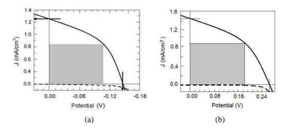
Fig. 14. Current-voltage characteristics of OSC-1(a): Pin = 56 mW/cm<sup>2</sup>, Voc = 0.14 V, Jsc =  $1.24 \text{ mA/cm}^2$ , FF = 0.53, PCE = 0.17% and OSC-2 (b): Pin = 56 mW/cm<sup>2</sup>, Voc = 0.243 V, Jsc =  $1.43 \text{ mA/cm}^2$ , FF = 0.64, PCE = 0.45 %.
