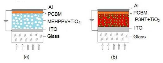
Fig. 11. Schematic drawing of OSCs based on nanocomposite of MEH-PPV+TiO<sub>2</sub> (a) and P3HT+TiO<sub>2</sub> (b). Thickness of the MTC and PTC layers is ~ 120 nm, PCBM layer -50 nm and Al-electrode - 70 nm.
