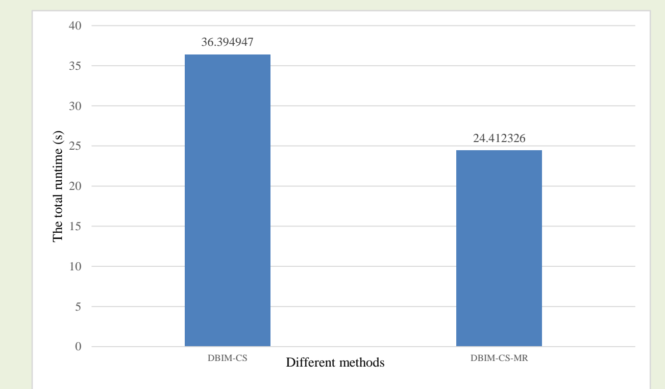
Fig. 6. The chart of the total runtime corresponding to different methods after N_{sum} iterations
