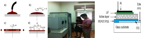
Fig 2. (a)- The spin-coating method; (b)- the sputtering method; (c)- the Organic Solar Cell
