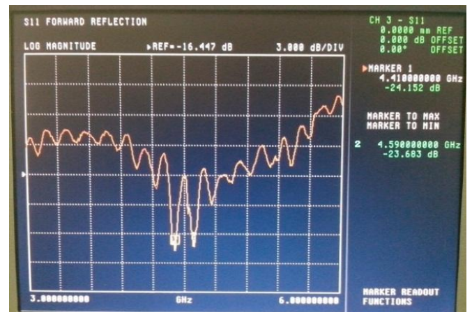
Figure 18: The input reflection coefficient S_{11}
