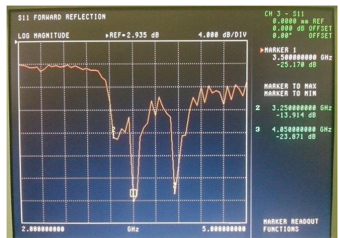
Figure 14: The input reflection coefficient S11
