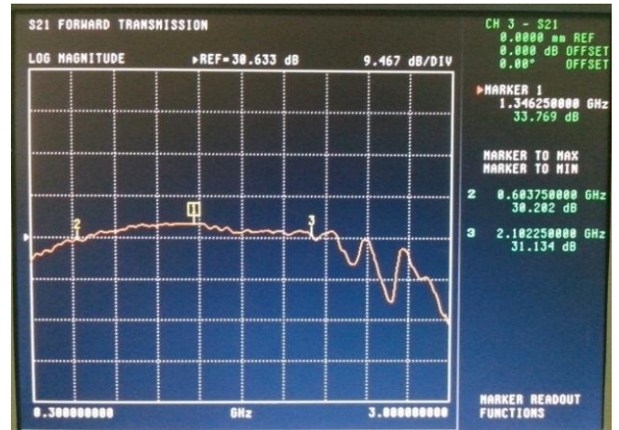
Figure 17: The gain of the IF amplifier
