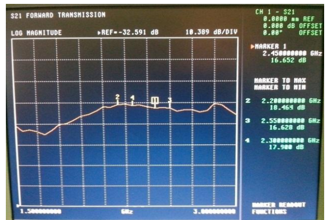
Figure 19: The gain of the VCO amplifier
