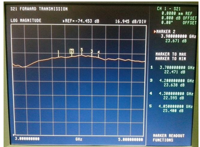
Figure 12: The gain of the LNA
