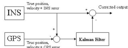
Figure 5. Feedforward configuration
