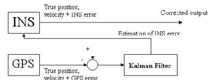
Figure 6. Feedback configuration
