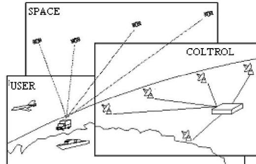
Figure 3. Structure of the GPS
