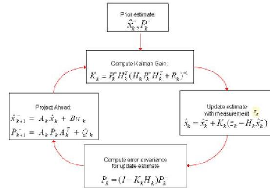
Figure 4. Kalman Filter loop
