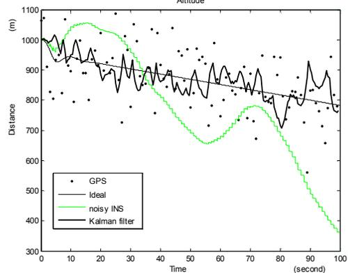
Figure 10. Altitude of the aircraft in case deviation of the GPS is increased.
