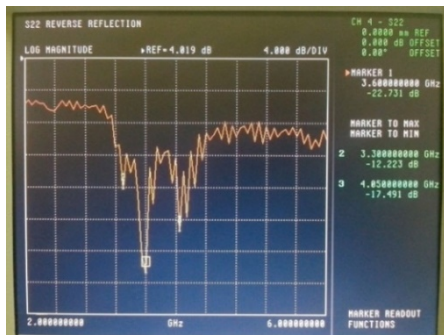
Figure 11. The output reflection coefficient S22
