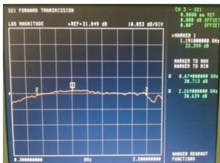
Figure 13. The gain of the IF amplifier
