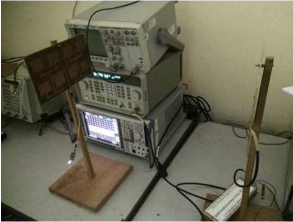
Fig. 13. Measurement setup for the WPT system.
