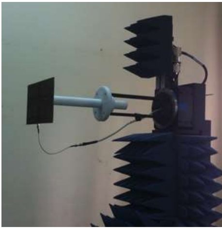
Fig. 10. The fabricated antenna measured by Nearfield System NSI 2000.
