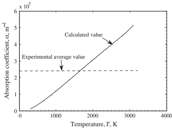
Fig. 5. Plot of absorption coefficient on the SiC surface as a function of temperature at nitrogen concentration of  $1.8 \times 10^{20} \text{ cm}^{-3}$ . Solid line represents the calculated results over the temperature range of 300–3100 K. Dashed line represents for the average value of absorption coefficient, which is predicted by experiment.
