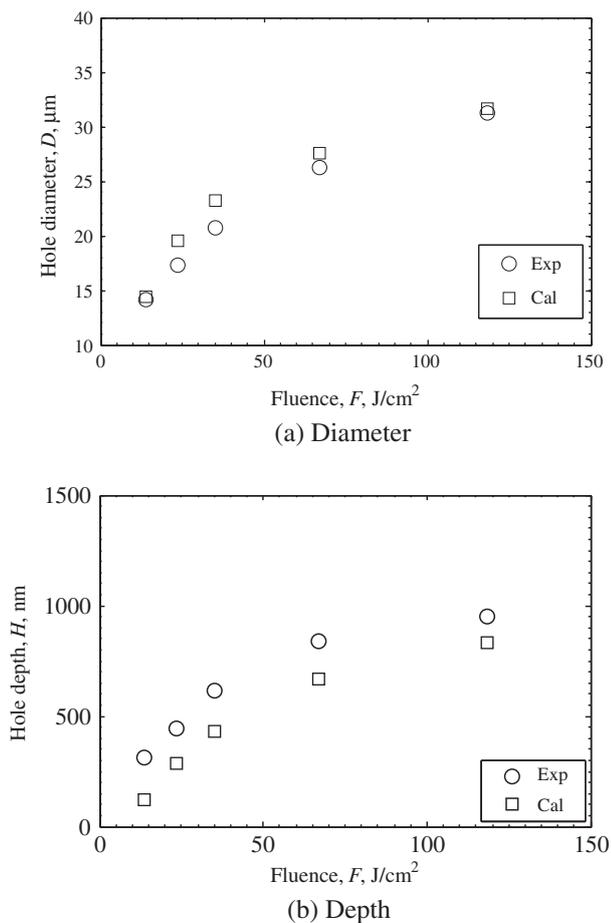
**Fig. 6.** Comparison of experimental and calculated diameter and depth of the ablated hole as a function of the fluence.
