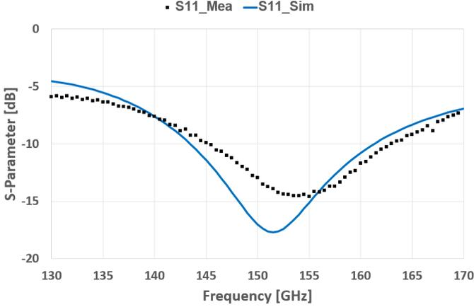
Fig. 4. The measured and simulated input return loss of the 300 GHz single varactor doubler.
