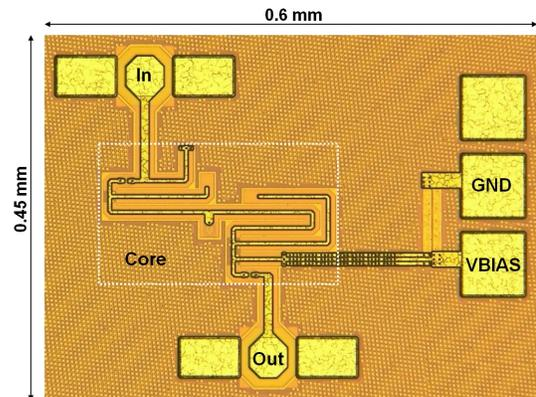
Fig. 3. The die microphotograph of the single varactor doubler.
