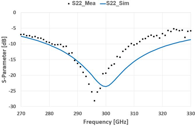
Fig. 5. The measured and simulated output return loss of the 300 GHz single varactor doubler.
