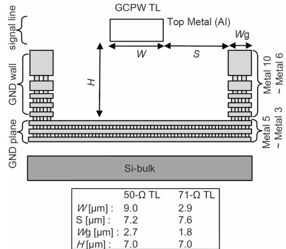
Fig. 1. The cross-view of the GCPW-TLs.
