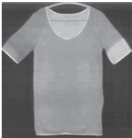
Fig. 4. The T-shirt dyed with the cationic dyes at ambient pressure showing color absorbance of the front side (treated surface) and the inside (non-treated surface).
