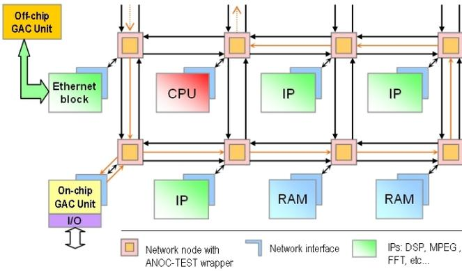
Fig. 3. ANoC-TEST general architecture.
