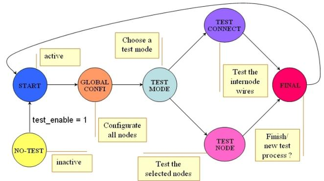
Fig. 5. The control flow of GAC unit.
