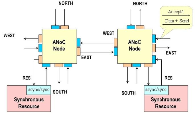
Fig. 2. Connections between two nodes.
