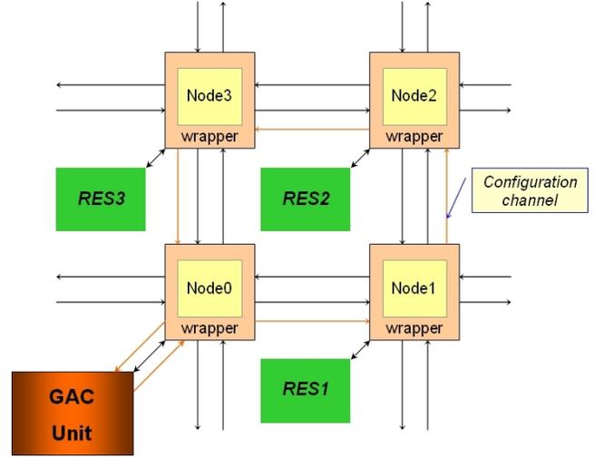
Fig. 6. A testbench with 4 asynchronous nodes and resources.
