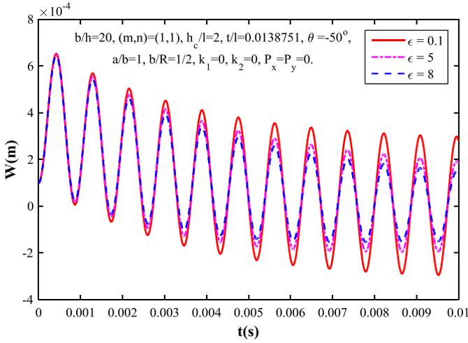
Fig. 10. Effect of damping coefficient  $\epsilon$  on the nonlinear dynamic response of the sandwich composite panels under blast loads.
