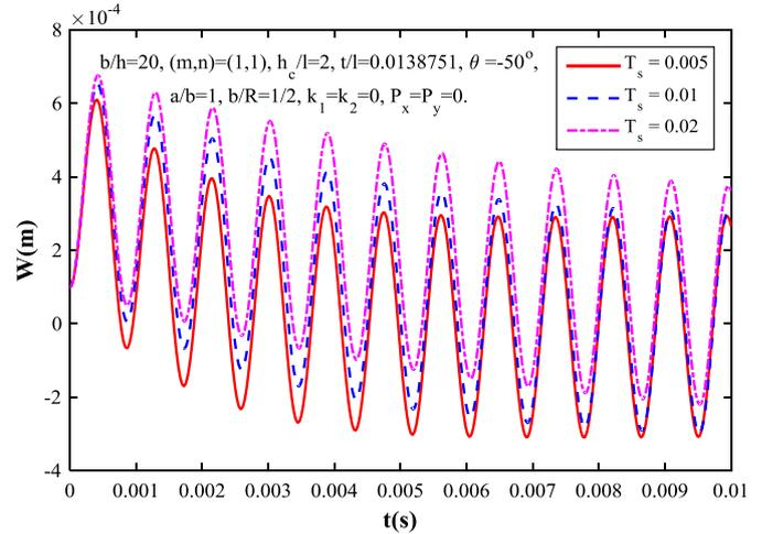
Fig. 8. Effect of parameter characterizing the duration of the blast pulse  $T_s$  on nonlinear response of the sandwich composite cylindrical panels.
