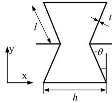
Fig. 2. Geometric of the cell of honeycomb core layer.
