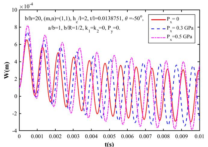
Fig. 9. Effect of pre-loaded axial  $P_x$  compression on nonlinear response of the sandwich composite cylindrical panels.
