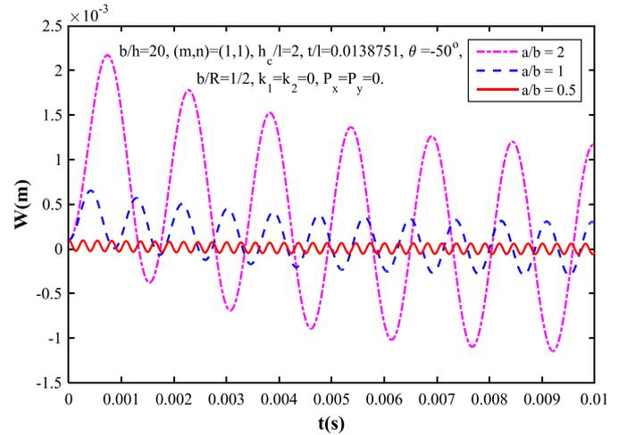
Fig. 4. Effects of ratio  $a/b$  on the nonlinear dynamic response of the cylindrical panels with negative Poisson's ratio in core layer under blast load.
