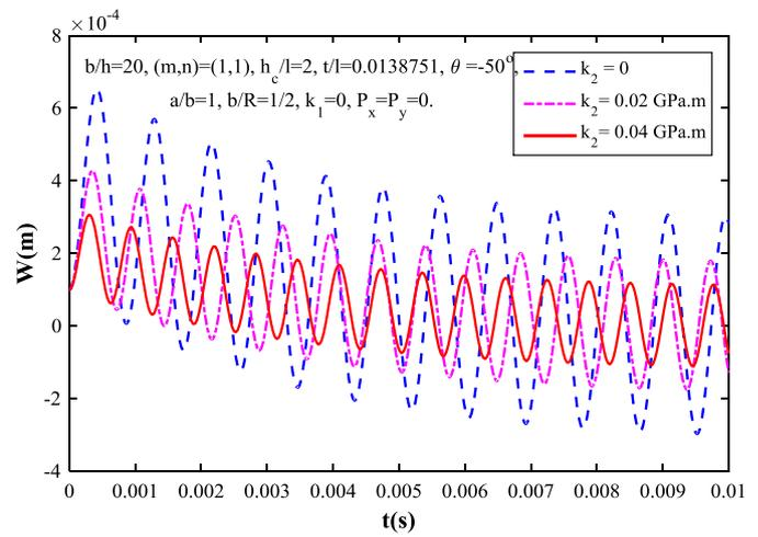
Fig. 7. Effect of the Pasternak foundation on the nonlinear dynamic response of the sandwich composite cylindrical panels.
