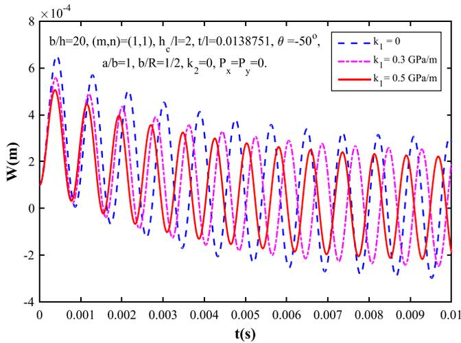
Fig. 6. Effect of the linear Winkler foundation on the nonlinear dynamic response of the sandwich composite cylindrical panels.
