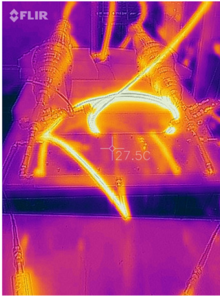
Fig. 11 Thermal image during high-power RF measurement. The Gysel combiner temperature is at 27.5°C. The maximum temperature is 45°C (yellow) and the minimum temperature is 25°C (purple)
