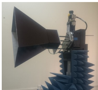
Figure 9. Measuring the antenna with NSI 2000 Near Field System
