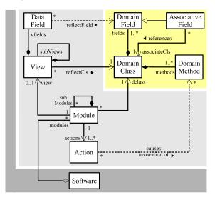
Figure 13: A high-level UML-based software model: (core layer) domain model, (middle layer) module, and (top layer) software.
