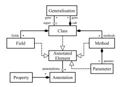
Figure 3: A high-level UML-based abstract syntax model of OOPL.
