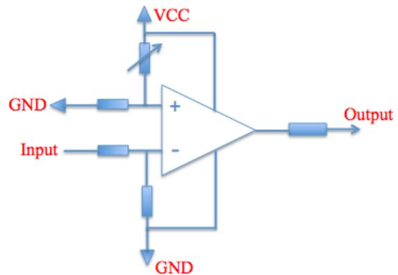
Figure 4. Working principle of the comparison amplifier
