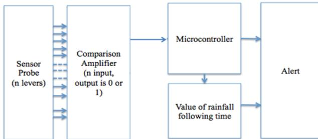
Figure 2. Electrode sensor interface with the MCU
