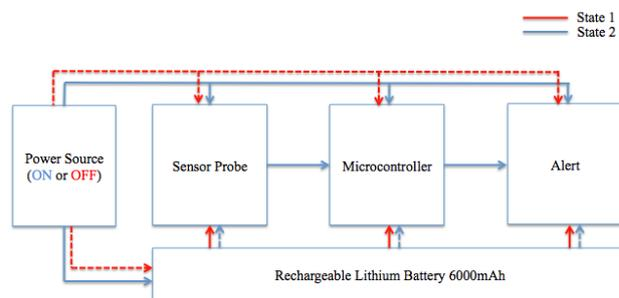
Figure 1. Block diagram of the device
