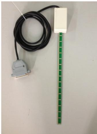
Figure 3. Photo of an electrode sensor
