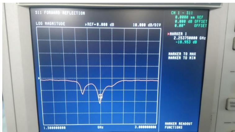
Figure 11. The measured  $S_{11}$  of the parallel coupled line microstrip bandpass filter
