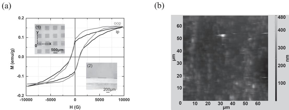
Fig. 3 (a) Magnetic hysteresis curves of squares. Inset: (1) surface and (2) cross-section image of squares. (b) Surface AFM image of one of squares.
