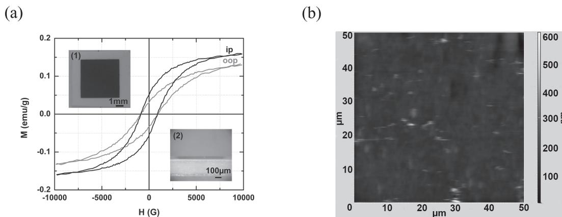
Fig. 2 (a) Magnetic hysteresis curves of  $5 \times 5 \text{ mm}^2$  film. Inset: (1) surface and (2) cross-section image of film. (b) Surface AFM image of film.
