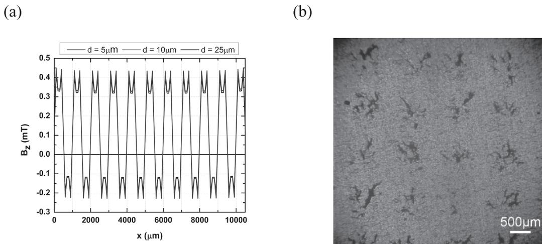
Fig. 4 (a) Magnetic induction ( $B_z$ ) at some heights ( $d$ ) on surface of squares along the  $x$  axis in inset (1) of Fig. 3(a). (b)  $Fe_3O_4$  particles in ferrofluidic solution attached to locations of squares under a Si sheet.
