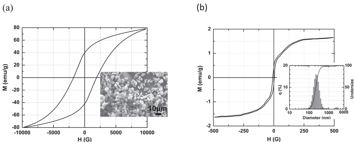
Fig. 1 (a) Magnetic hysteresis curve of Nd-Fe-B initial particles (inset: SEM image of initial particles). (b) Magnetic hysteresis curve of magnetic ink (inset: the particles size distribution of magnetic ink).
