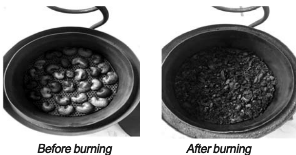
Figure 5: Procuduce charcoal from cashew nut shell
