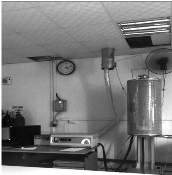
Figure 7: Pyrolysis experiments with Macro TG machine
