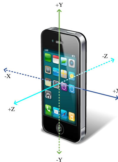
Figure 2: Three-axis accelerometer of a smartphone.
