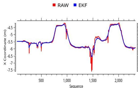
Figure 6. Illustration of using the EKF to estimate the position on the X axis
