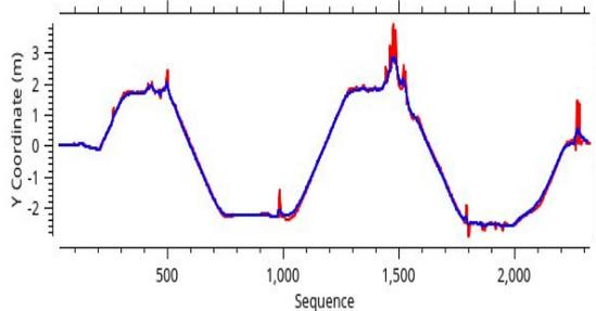
Figure 7. Illustration of using the EKF to estimate the position on the Y axis
