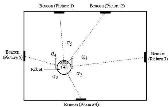
Figure 1. Robot Get Positions with IPS Beacons
