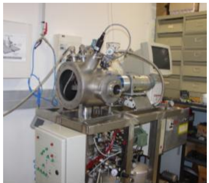
Fig. 1 : The general view of tribometer pion-disc type (disc support, chamber, vacuum pump)
