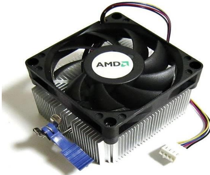
Figure 5. Combination of an aluminum sheet and a fan for cooling system
