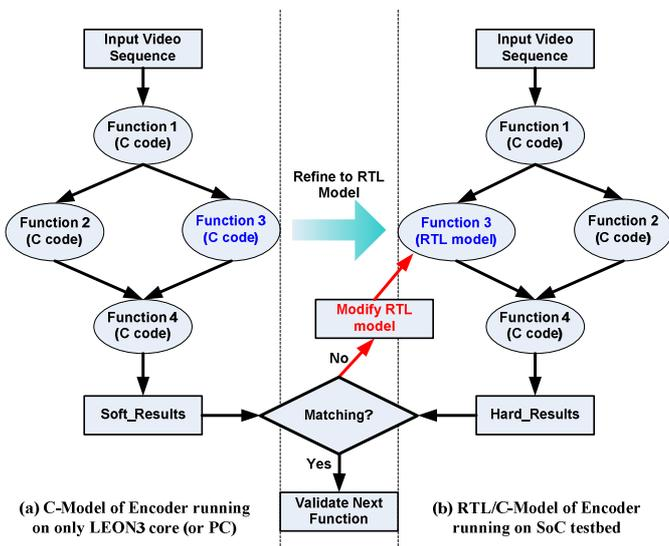
Fig. 5. Method for validating the RTL design on the SoC testbed.
