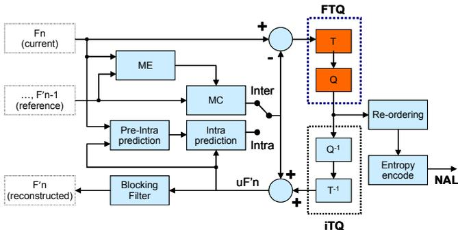
Fig. 1 Functional diagram of the H.264/AVC encoder.
