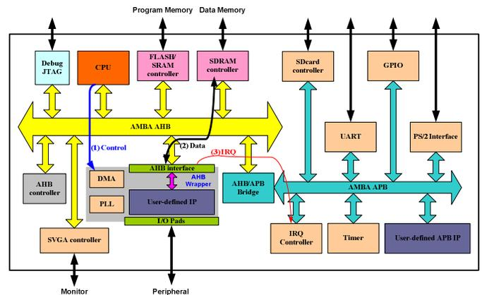
Fig. 6. The process of validating one IP core on the emulation board.
