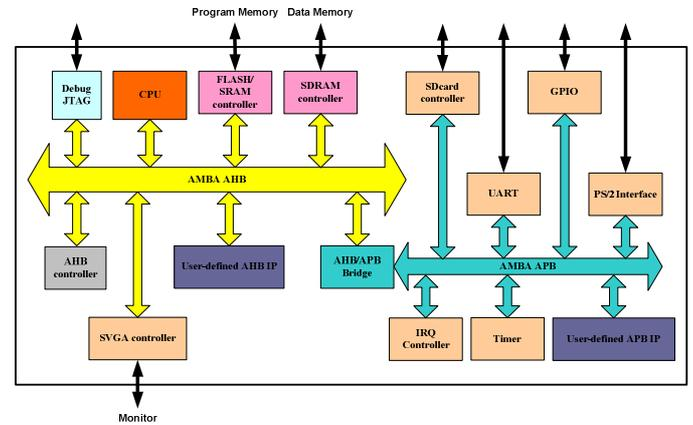
Fig. 3. Top-level architecture of SoC testbed.
