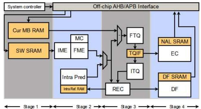
Fig. 2 VENGME H.264/AVC encoder architecture.
