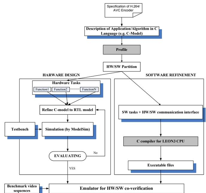
Fig. 4. Design and verification flow.
