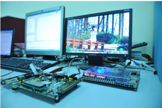
Fig. 8. Testbed implementation on Altera DE2 development board.
