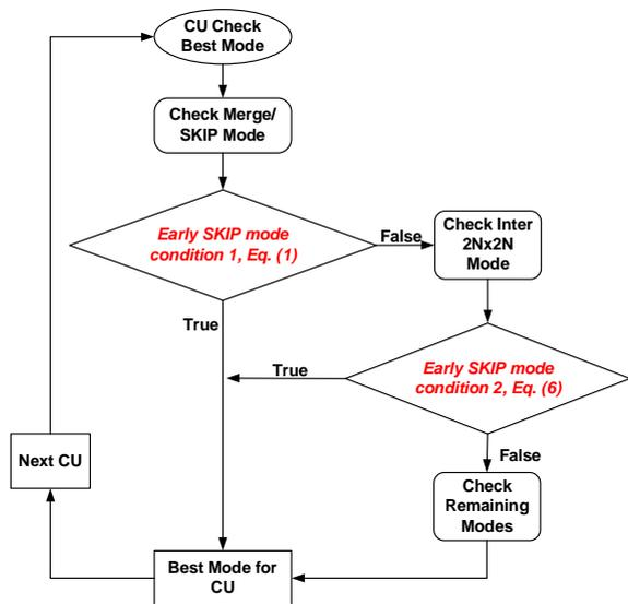
Figure 6. Proposed fast HEVC inter coding (CU: Coding Unit)
