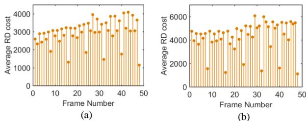
Figure 5. The average RD-cost of the SKIP mode in each frame in sequence (a) BQMall, (b) Racehorses
