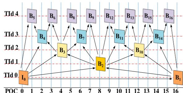
Figure 2. HEVC hierarchical coding structure
