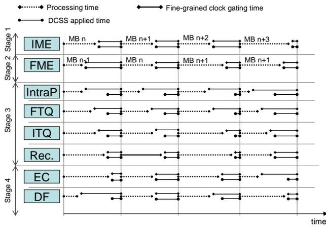
Figure 4. DCSS [16] and fine-grained clock gating [9] exploit schedule of H.264 encoder.
