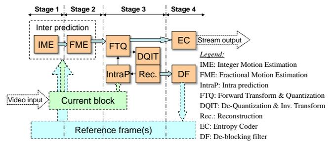
Figure 2. Classical 4-stage pipeline architecture of H.264 hardware encoder.
