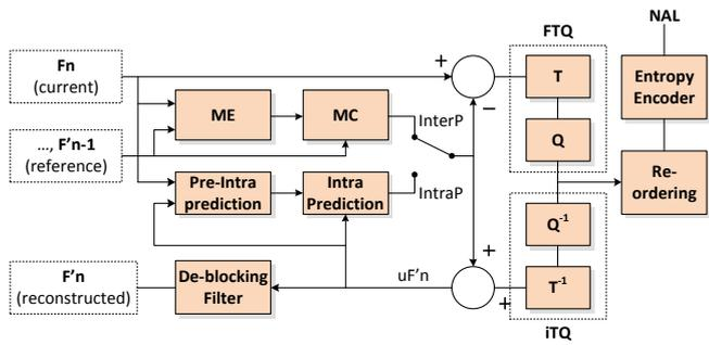
Figure 1. Functional diagram of the H.264/AVC encoder.
