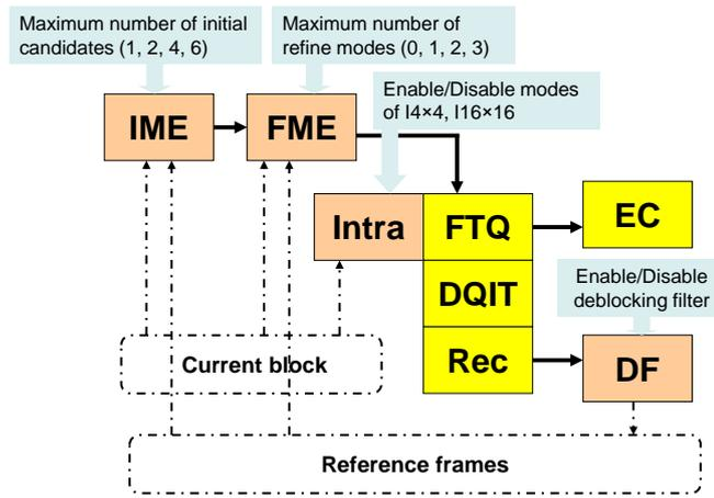
Figure 5. Parameterized video encoder.
