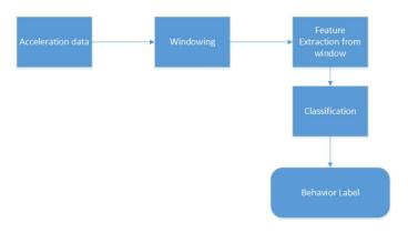
Figure 2. Behavior recognition process pipeline.
