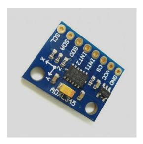
Figure 4. Acceleration sensor ADXL345.
