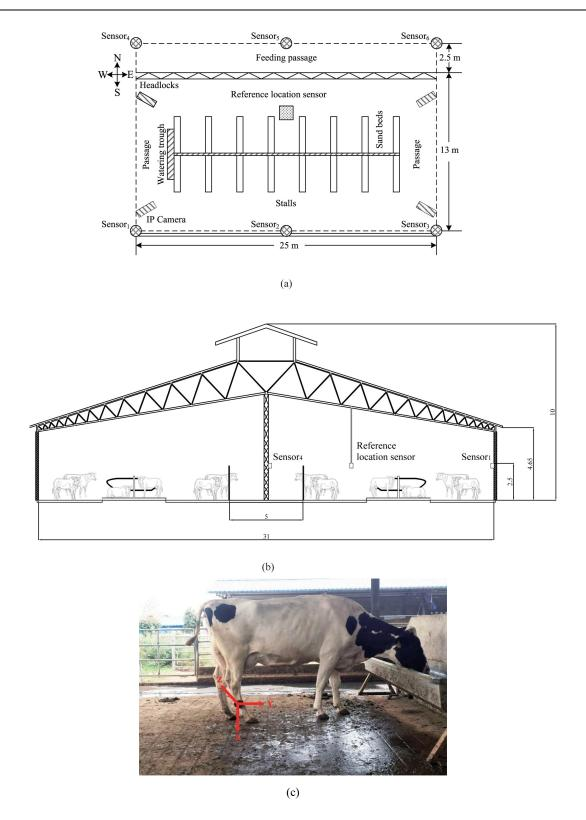
**Figure 1.** Plan and section of the studied area in the barn [20]. (a) Plan. (b) Section. Sensor is attached to the leg of a cow. (c) Copyright: © 2018 Wang et al. [20].
