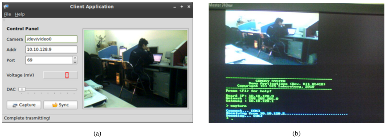
Figure 7. Validation results: (a) Client application view on PC side with captured image and other parameters; (b) Embedded application view on CoMoSy side with decoded image.
