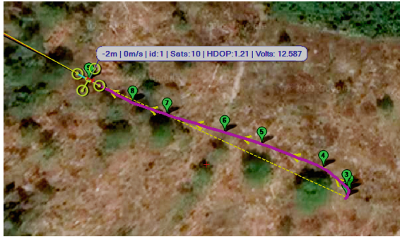
Fig. 6. The real flight path (solid purple line) overlapping the planned path (solid yellow path with arrows)
