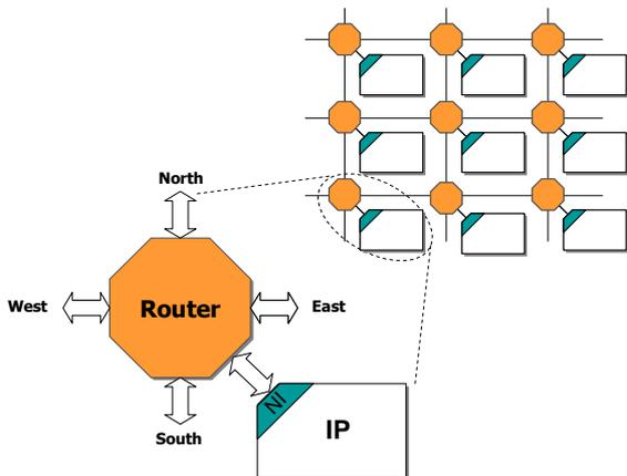
Figure 1: 2-D mesh NoC architecture.
