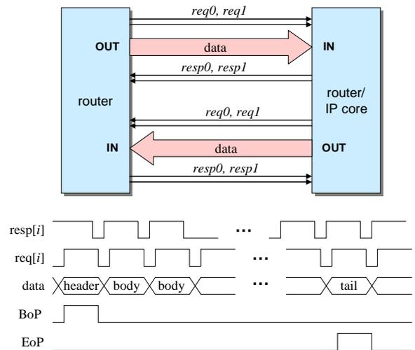
Figure 3: Router-to-router/IP core interface and handshake protocol.
