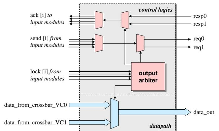
Figure 6: Micro-architecture of output module (OM).
