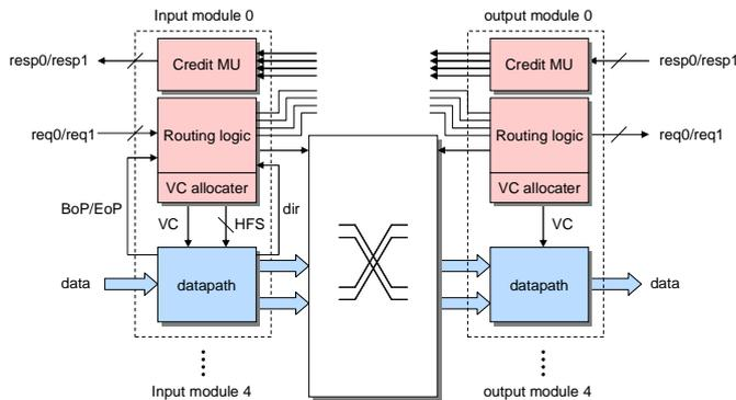
Figure 4: Router architecture.
