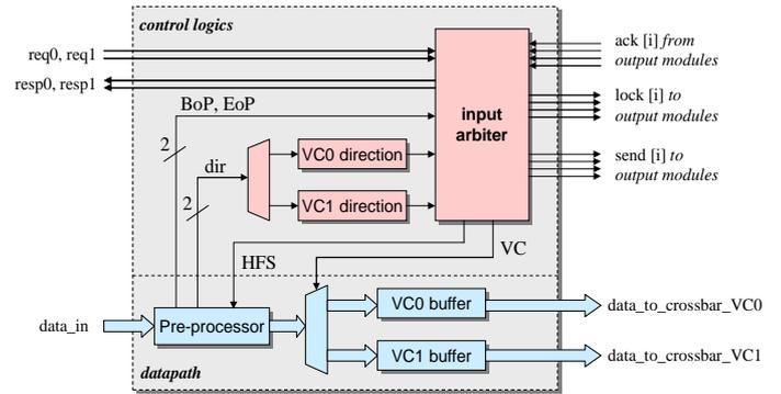
Figure 5: Micro-architecture of input module (IM).
