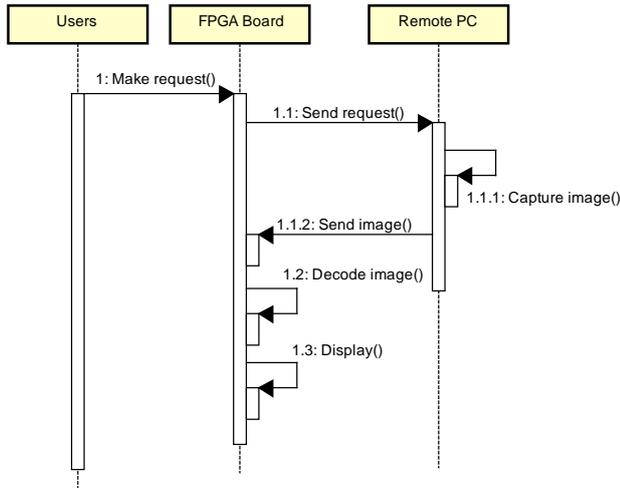
Fig. 8. Sequence diagram of the remote camera system.
