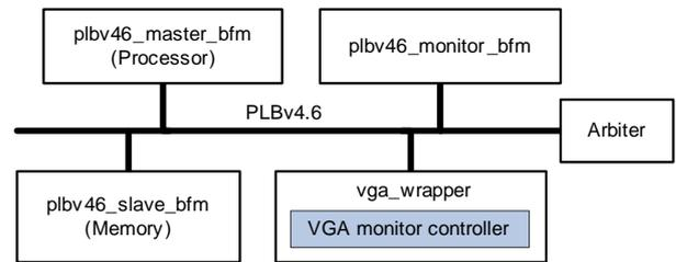
Fig. 5. Verification model for VGA monitor controller.
