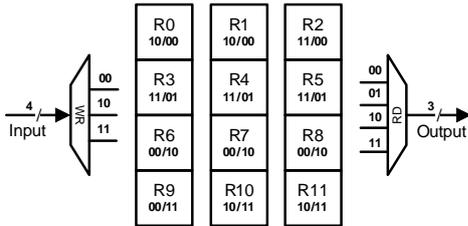
Fig. 2. VGA Data Aligner for 32 bits mode.
